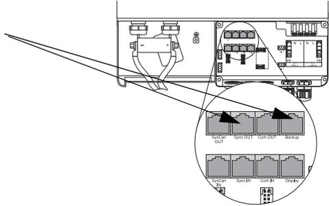
5. If applicable, install the communication cables of the external communication device (see section 7.5.2 „SBU 2200 and an External Communication Device“ (62)) before assembling the feed-through element and then re-inserting it into the installation opening on the Sunny Backup 2200.
