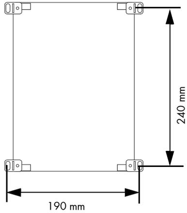
4. Mark drill holes on the wall.
