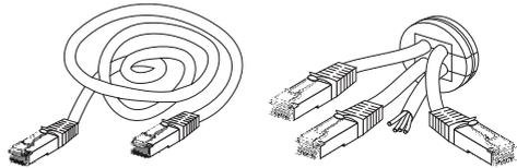
4. Install all communication cables (see section 7.5 „Communication“ (61)) before assembling the feed-through element and then re-inserting it into the installation opening on the Sunny Backup 2200.
