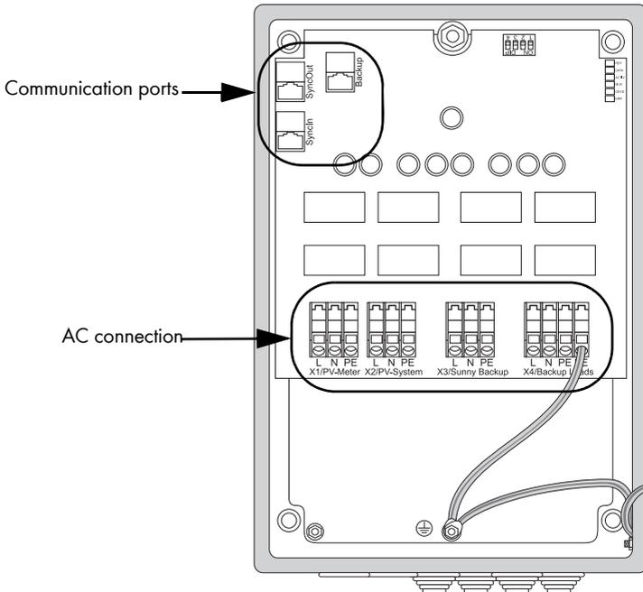
All cables are fed into the housing from underneath.
