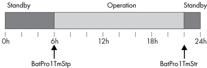
**Level 2:** The second level of the battery preservation mode ensures that the Sunny Backup 2200 regularly starts every two hours, but only during the window of time in which an energy supply is expected, and attempts to charge the battery from the AC side. For photovoltaic systems, this occurs during the day. In this case, you define the start time using the "223.03 BatPro2TmStr" parameter and the stop time using the "223.04 BatPro2TmStp" parameter.
