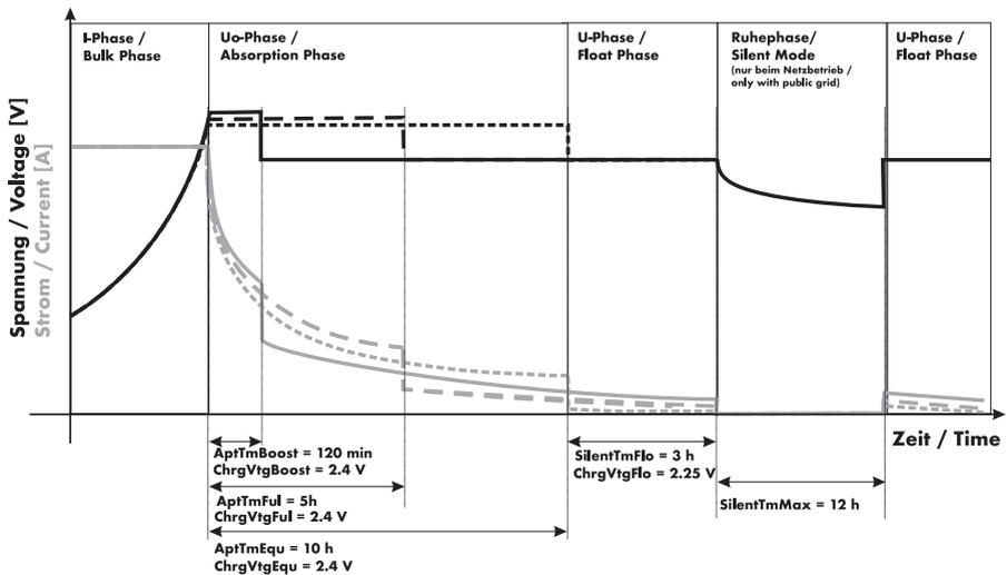
The I stands for the constant voltage phase (I phase). In this phase, the charging process is limited by the maximum specified battery current ("222.01 BatChrgCurMax" parameter), the nominal grid current ("232.03 GdCurNom" parameter) or the maximum AC charging current of the Sunny Backup 2200 ("210.02 InvChrgCurMax" parameter). The respective value reached first is the limiting value. During this phase the battery voltage increases as the battery is charged.
