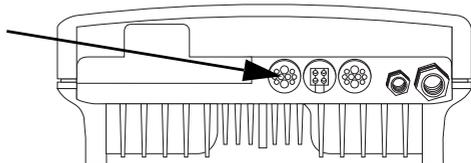
4. Insert one wire into each "BatTmp" connection terminal of the 4-pole print terminal included in the delivery.
