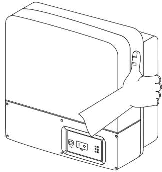
3. Attach the device to the wall mounting bracket slightly to the left using its mounting plate. The right edge of the rear wall of the device must be flush with the right edge of the wall bracket.
