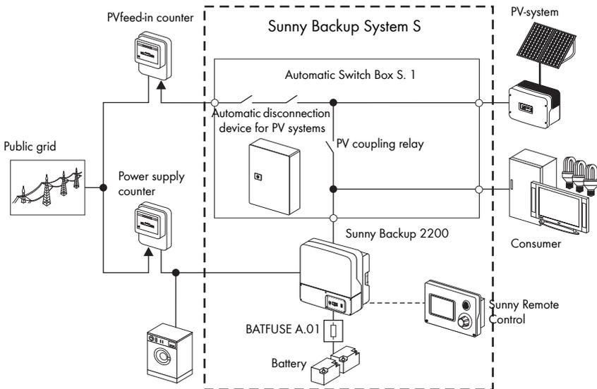
The Sunny Backup System S is suitable for use in conjunction with the Sunny Boy PV inverters from SMA Solar Technology AG. The Sunny Backup System S can be integrated into new PV system installations, and can also be retrofitted onto existing PV systems.
