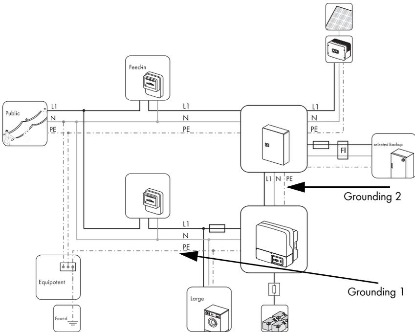
1. The first ground connection is made using the protective earth conductor from the PV feed-in counter to the Sunny Backup 2200 via the Automatic Switch Box S.
