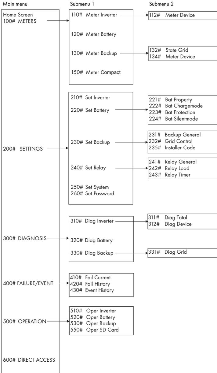
Only parameters in the menu branches "200# Settings" and "500# Operation" can be changed. All other values are only displayed. All menu items that can only be changed after entering the installer password are shaded in gray in the following tables.
