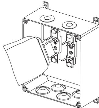
8. Now quickly push the NH fuse into the bracket.
