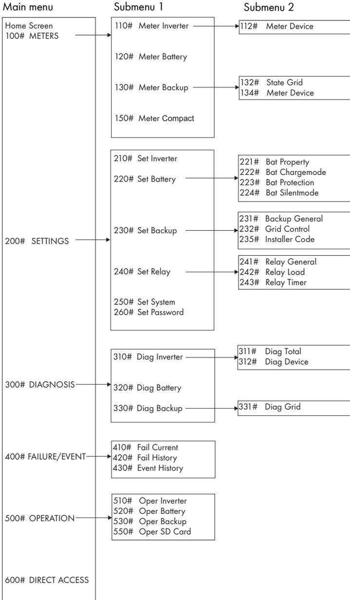
**100# Meters - Display values:** This menu contains the display values for the following backup system components:
