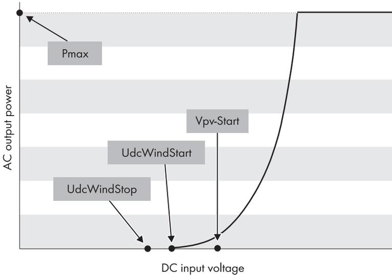
Figure 9: The feed-in AC power in relation to the inverter's DC input voltage.
