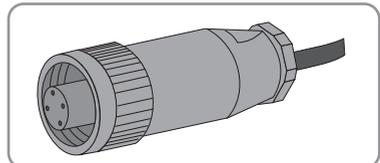
12. If the cable diameter is between 13.5 mm ... 17 mm, tighten the cable gland lock nut firmly on the threaded sleeve.
