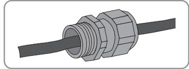
8. Pass the threaded sleeve over the AC cable.
