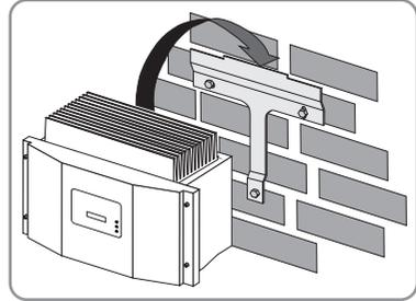
4. To secure the inverter from lifted out, fasten the inverter on the wall mounting bracket using the provided M6x12 cylinder head screw.
