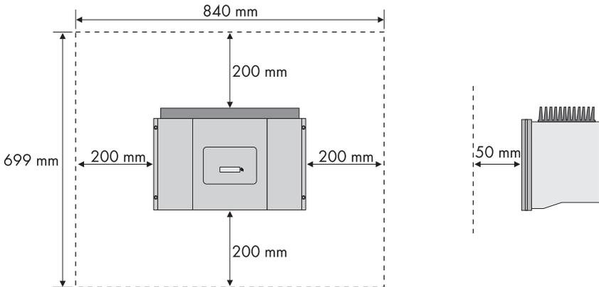
Figure 3: Minimum clearances to be observed
