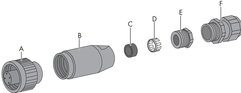
Figure 8: AC plug components (included in delivery)
