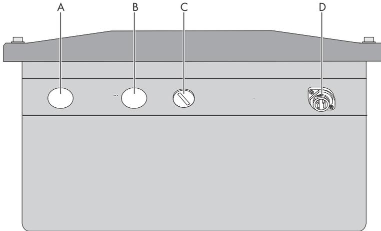
Figure 6: Enclosure openings and plug at the bottom of the inverter
