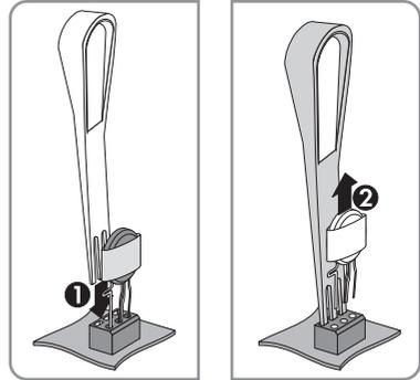
5. Insert new varistor. Insert the loop or crimp into the outer terminal (see "Position of Varistors", page 33).
