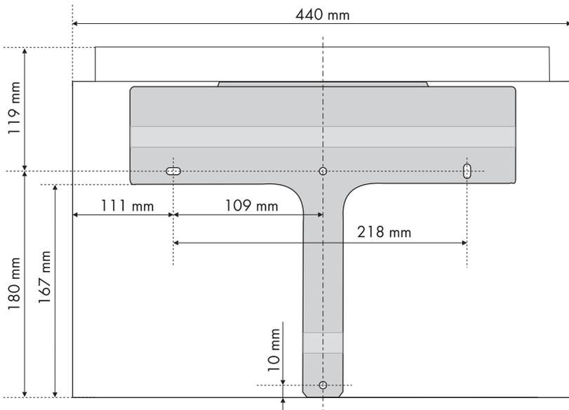
Figure 5: Wall mounting bracket dimensioning
