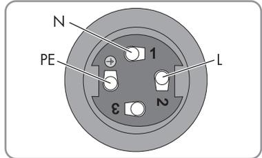
10. Check that the PE, N and L are securely in place.
