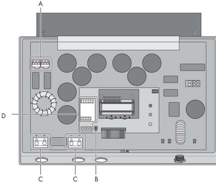
Figure 7: Connections inside the inverter
